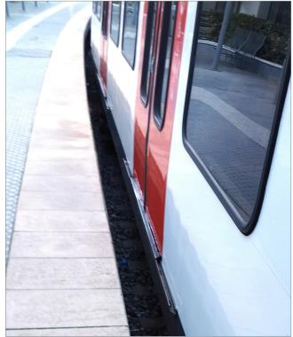
The **Gap-Fille**r is an automatically extending board that provides a safe and comfortable passenger access, especially for people with reduced mobility.
